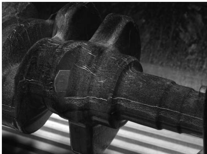
FIG. A1.4 Crankshaft with Various Longitudinal Indications
